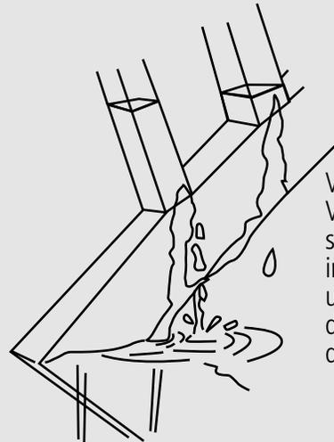
Vent and drain hole size. Vent and drain holes that are too small in hollow sections increase immersion time and may cause unsightly excessive zinc drainage runs as the zinc freezes during the draining period.
