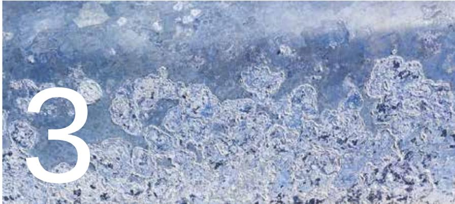
**Photo 3** : Example of white corrosion on a galvanized surface.
