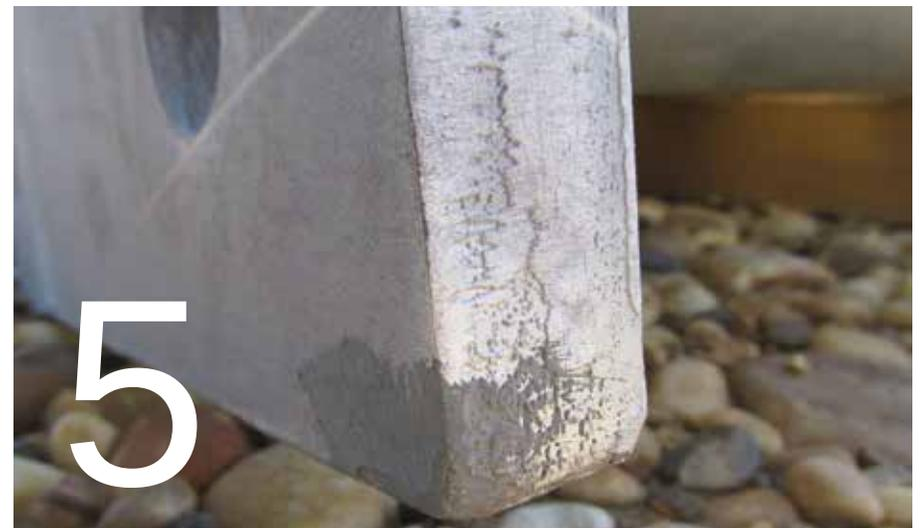
**Photo 5** : Example of galvanized material repaired with zinc paste.
