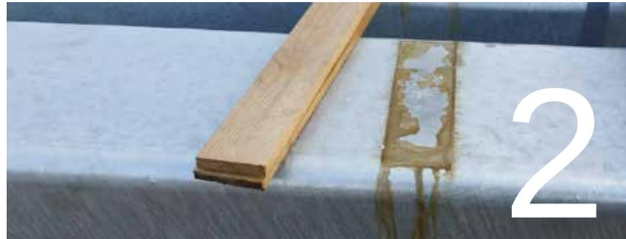
**Photo 2 :** Example of marks left on zinc by contact with wood whose sap is acidic.
